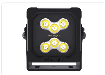
Piranha 6. Six LEDs, 55 W, 6,300 lumens, 9 to 35 VDC for 12 and 24 V machines, drivers on board. DC only, PIDC01
