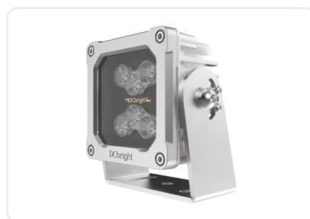
Piranha SS. The 9 and the 6 in solid 316L stainless steel, electrolytically polished, glass front, twenty years on the housing. PISS01 and PISS02
