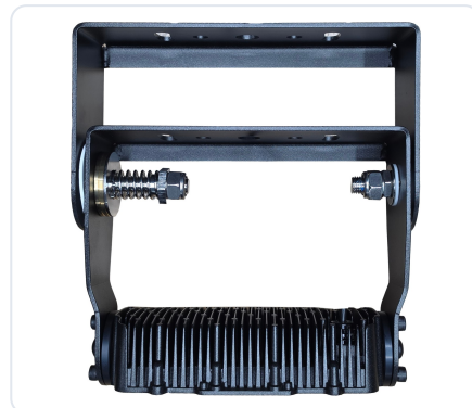
Crane Light Stabilizer. For a crane boom. The swing arm keeps the luminaire level while the boom moves. Separate datasheet
