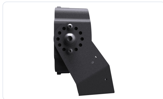
The detent ring: twelve holes, a central pivot bolt and two index bolts. Twelve holes is where 30 degrees comes from
