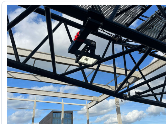
Shark on the Crane Light Stabilizer, mounted on a lattice jib.
