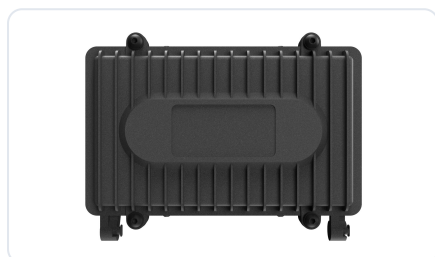
DRB-1. One driver up to 320 W in a finned aluminium box, IP66 and IP67, 4.2 kg. Wall, pole or rear mounted. The standard box for one floodlight
